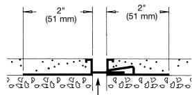
Adjusts from 0" to 1/2" (0-13 mm)
