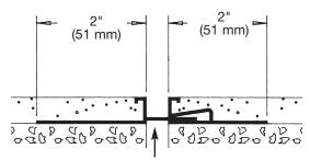
Adjusts from 0" to 1/2" (0-13 mm)
