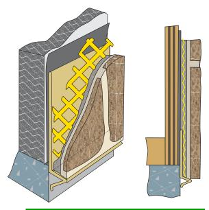
All butt joints, intersections and ends shall be caulked at the time of installation using an elastomeric sealant, such as Plastic Components' Ultra-Tech™ (PC-ULTW).
