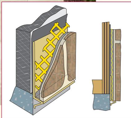
They provide a stop for stone veneer and allow moisture to migrate down and away from the wall.
