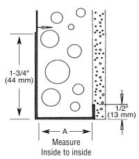
Add suffix "WP" to order with weep holes. Example: CBWP-15-16 - 10' (3 m) Lengths \*Dimension "A"- measure inside to inside
