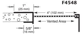
The base coat mesh should be lapped over the top of the perforated flanges and across all butt joints.
