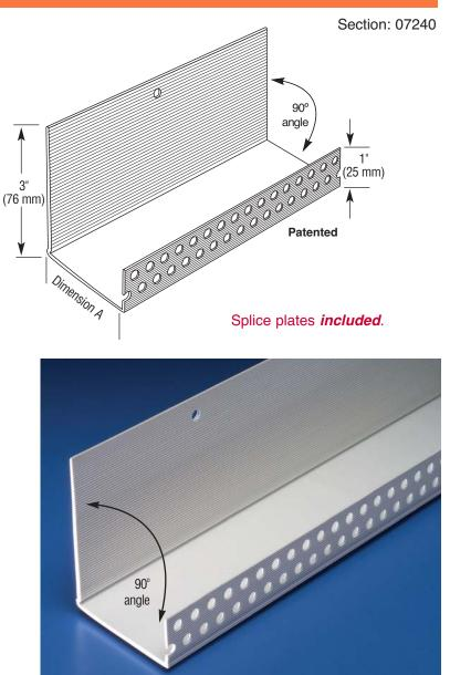
Application: Can be used as a STARTER TRAC® at the base of a wall or an EIFS Casing Bead around window and door openings. Face return flange is 1" (25 mm) with striations which provide a strong physical bond for the base coat and perforations for bonding the base to the substrate. Available with weep holes. Ideal for use where finished edge is exposed. 3" (76 mm) wide nailing flange also has striations for extra bonding.
