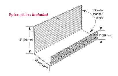
**Application:** Can be used as a STARTER TRAC® at the base of a wall or an EIFS Casing Bead around window and door openings. Face return flange is 1" (25 mm) with striations which provide a strong physical bond for the base coat and perforations for bonding the base to the substrate. Available with weep holes. Ideal for use where finished edge is exposed. 3" (76 mm) wide nailing flange also has striations for extra bonding.
