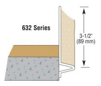
All butt joints, intersections and ends shall be caulked at the time of installation using an elastomeric sealant, such as Plastic Components' Ultra-Tech™ (PC-ULTW).
