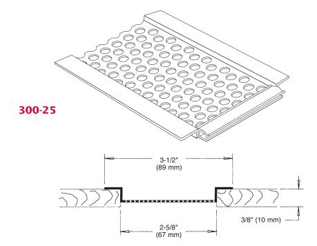
Note Caulk all butt joints, ends, angles, corners, and intersections at time of installation.
