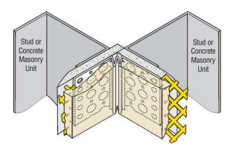
All butt joints, intersections and ends shall be caulked at the time of installation using an elastomeric sealant, such as Plastic Components' Ultra-Tech $^{\text{TM}}$  (PC-ULTW).
