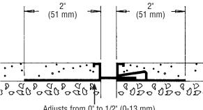
Adjusts from 0" to 1/2" (0-13 mm)
