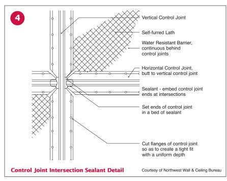
Caulk all butt joints, intersections and ends at time of installation using an elastomeric sealant such as Plastic Components' Ultra-Tech™ (PC-ULTW)
