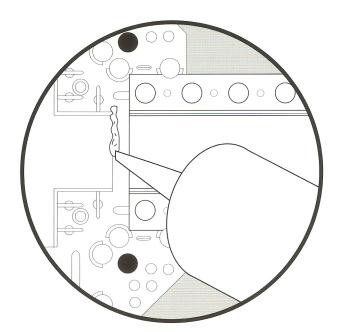
3) Apply a bead of caulk at the connecting point to ensure a positive water seal. Remove excess caulk with a clean rag.
