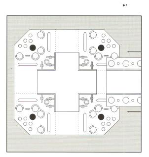
2) Insert ULTRA-TRAC<sup>®</sup> reveal into the intersection under the alignment guides. Prior to final placement of reveal...
