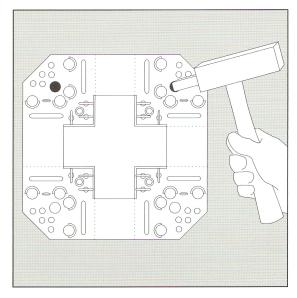
1) Attach ULTRA-TRAC® intersection to substrate at pre-determined location.
