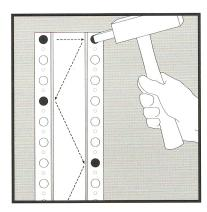
Attach alternate sides at 8" intervals, while keeping reveal level and straight.
