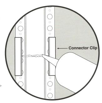
For continous application (horizontal or vertical). Use a connector clip to join ends together. Apply a bead of caulk to the seam. Remove excess caulk with a clean rag. All surfaces must be free of oil, dirt and other foreign material. Clean **only** with soap and water.
