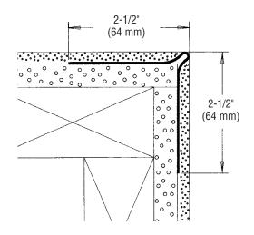
The base coat mesh should be lapped over the top of the perforated flanges and across all butt joints.
