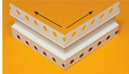
The base coat mesh should be lapped over the top of the perforated flanges and across all butt joints.
