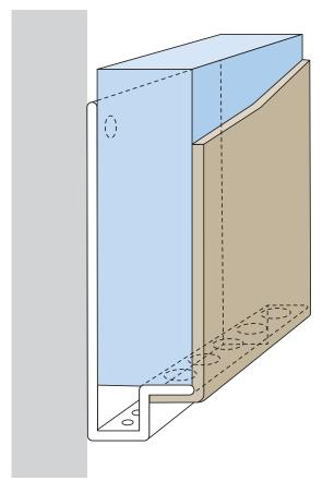
The base coat mesh should be lapped over the top of the perforated flanges and across all butt joints.
